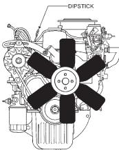
Figure 13. Engine Oil Dipstick (Removal)
